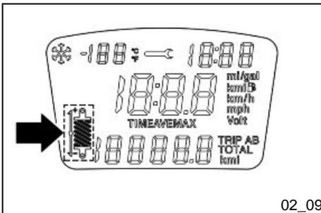
The greater the number of turns shown, the lower the preloading of the shock absorber:
