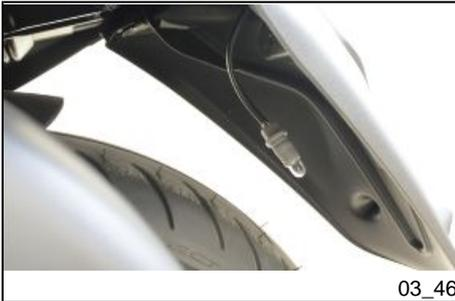
Replace the license plate light bulb by sliding it off from the bulb holder.
