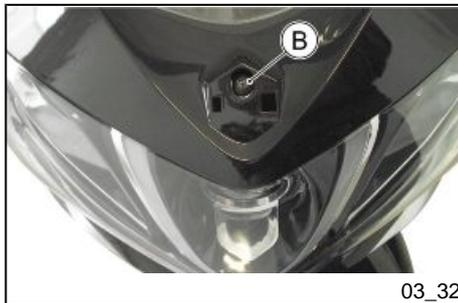
Unscrew and remove the front screw «**B**».
