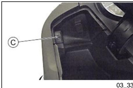
Turn the handlebars to the side opposite to the one on which you are operating and, after lifting the door of the respective dashboard glove-box, unscrew the screw «**C**», first operating on the left side and then on the right side of the vehicle.
