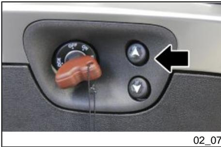
Press on the «**UP**» and «**DOWN**» buttons, after setting the key to «**ON**», to increase or decrease the rear shock absorber preloading.
