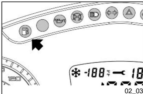
The reserve fuel level is indicated by the warning light on the instrument panel turned on.
