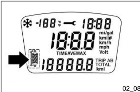
On the display the preloading is visualised via the indicated icon.
